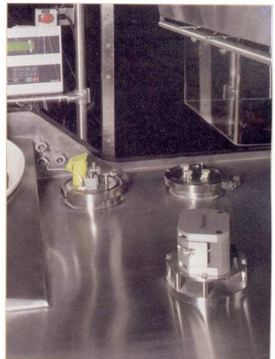
Peristaltic pump is easily integrated into the work surface of IsoTech aseptic filling isolator
