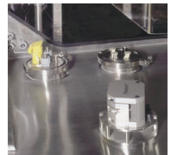
FLEXICON PERISTALTIC PUMP AND SANITARY CONNECTIONS INTEGRATED IN WORK SURFACE OF ISOSPHERE™-AF
